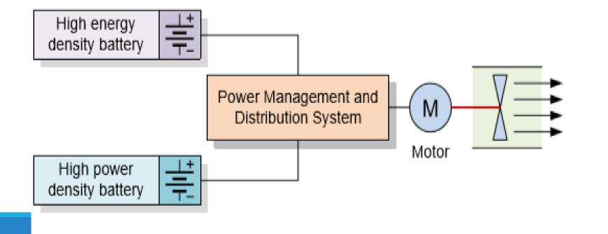
6. Battery System Design for high specific power and energy [27].
